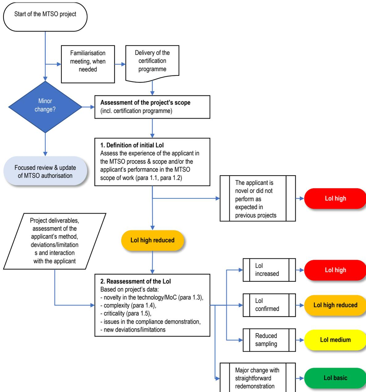
**Figure 1: Process of determination of the Authority's Lol in MTSO certification projects**
